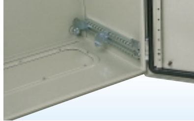
Movable plate support with positions every 12.5 mm. Front part has M6 ø drill holes to enable various items to be fitted.
