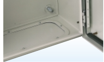
Close up of back of enclosure with 4 M8 x15 welded studs for fixing the mounting plate, and wall fixing holes closed with plastic plugs.
